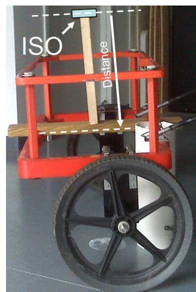
FIGURE 1-6 Example Spike Test Setup
