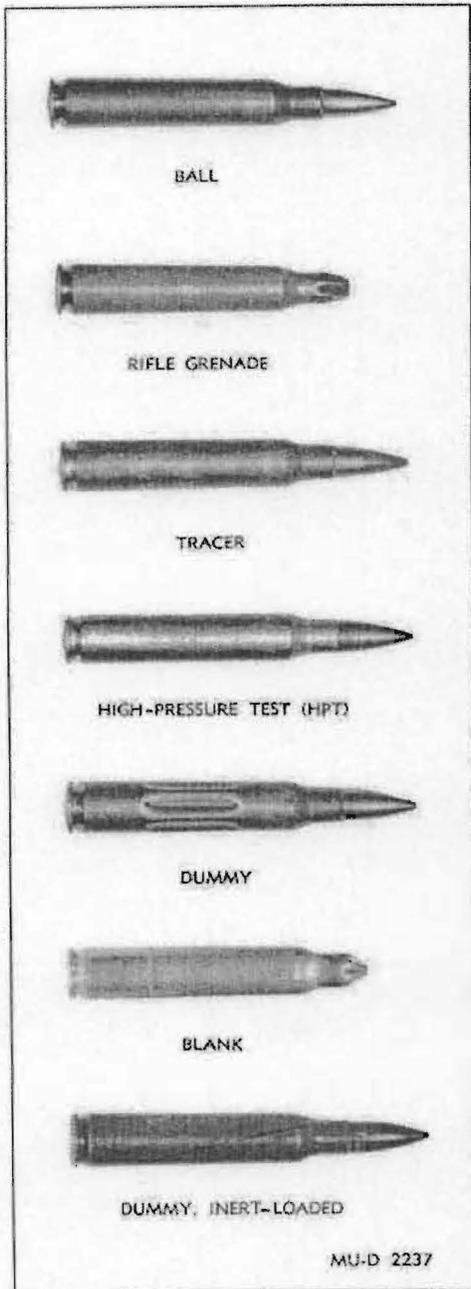
Figure 6. 5.56mm cartridges
