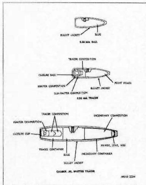
Figure 3. 5.56mm and caliber .50 spotter tracer bullets (sectional)
