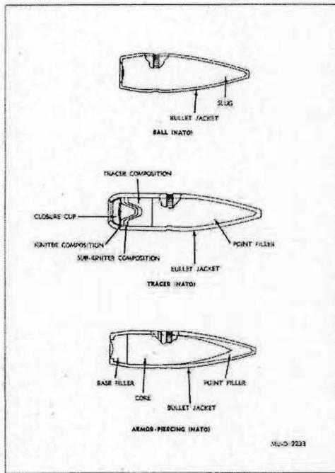
Figure 2. 7.62 mm bullets (sectional)
