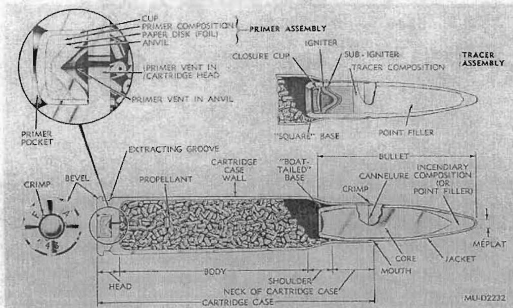
Figure 1. Typical cartridge (sectional)
